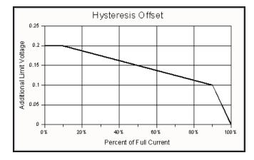
The limit current circuit contains a small amount of hysteresis, which causes the limit current to trip slightly before expected. If the PLD current is close to the limit setpoint this hysteresis may affect operation. To compensate, a small offset voltage can be added to the limit current setting based on the Hysteresis offset chart above.
