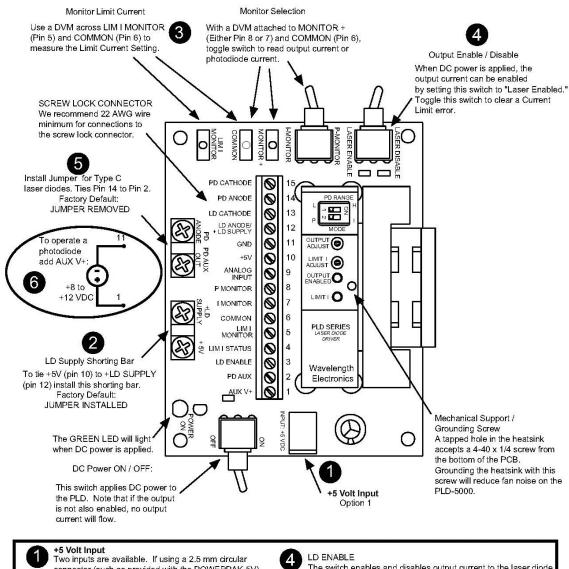
Two inputs are available. If using a 2.5 mm circular connector (such as provided with the POWERPAK-5V) use the DC input next to the power switch. Otherwise, use the screw-lock connector, pins 10 & 11.
